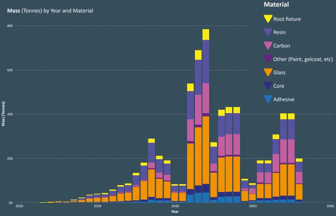
Figure 4 Offshore blade masses by material
